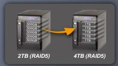
The storage capacity of a RAID configuration can be expanded by replacing the hard drives with larger ones. All the data will be kept and seamlessly moved to the newly installed hard drives. There is no need to turn off the server during the process.
